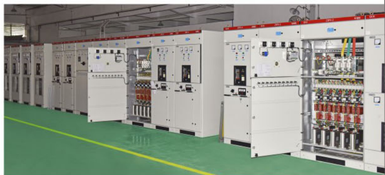
高低压柜生产车间 | High and low voltage cabinet production workshop |
